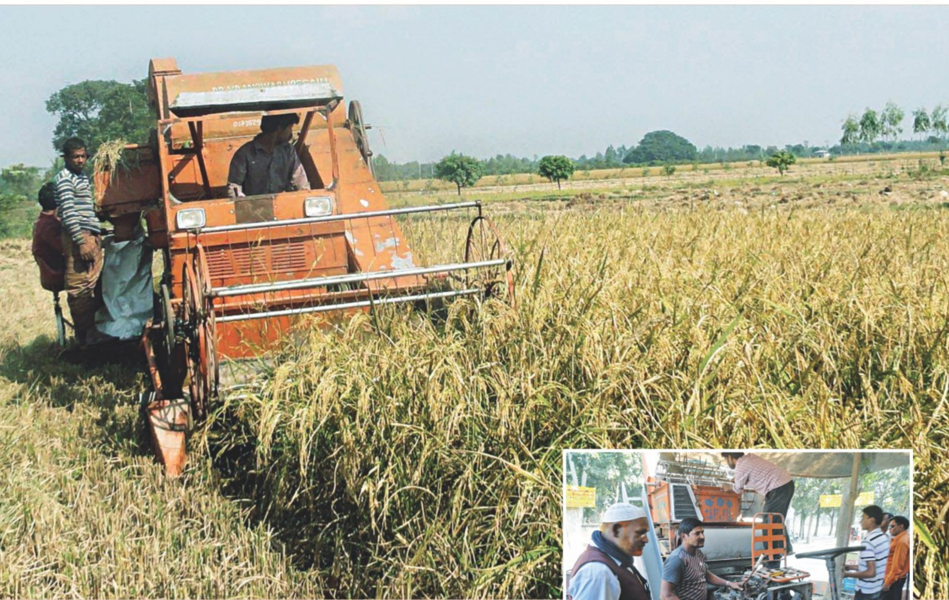
The locally made machine, which can harvest one acre per hour, is in operation in a paddy field of Dinajpur. Inset, Anwar Hossain, the designer of the machine, and his assistants are busy developing a new device at his workshop.
