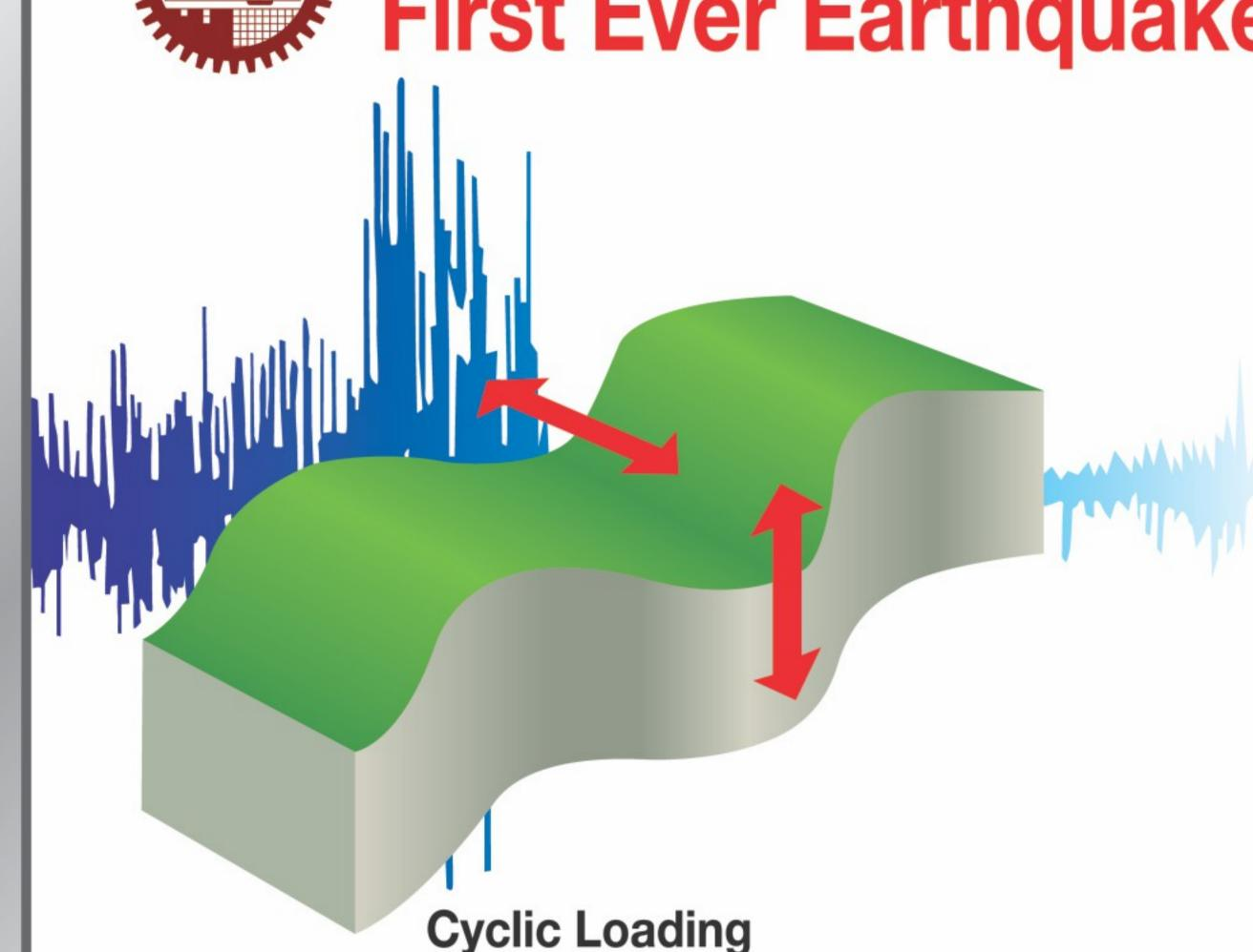
Strength and Ductility are essential qualities of construction steel but they are not sufficient in a disaster like earthquake. During a laboratory test, strength and ductility of steel are examined by applying uni-directional load. In the event of an earthquake, the force unleashed is multi-directional and creates both horizontal & vertical bending stress on structures, known as cyclic loading.
