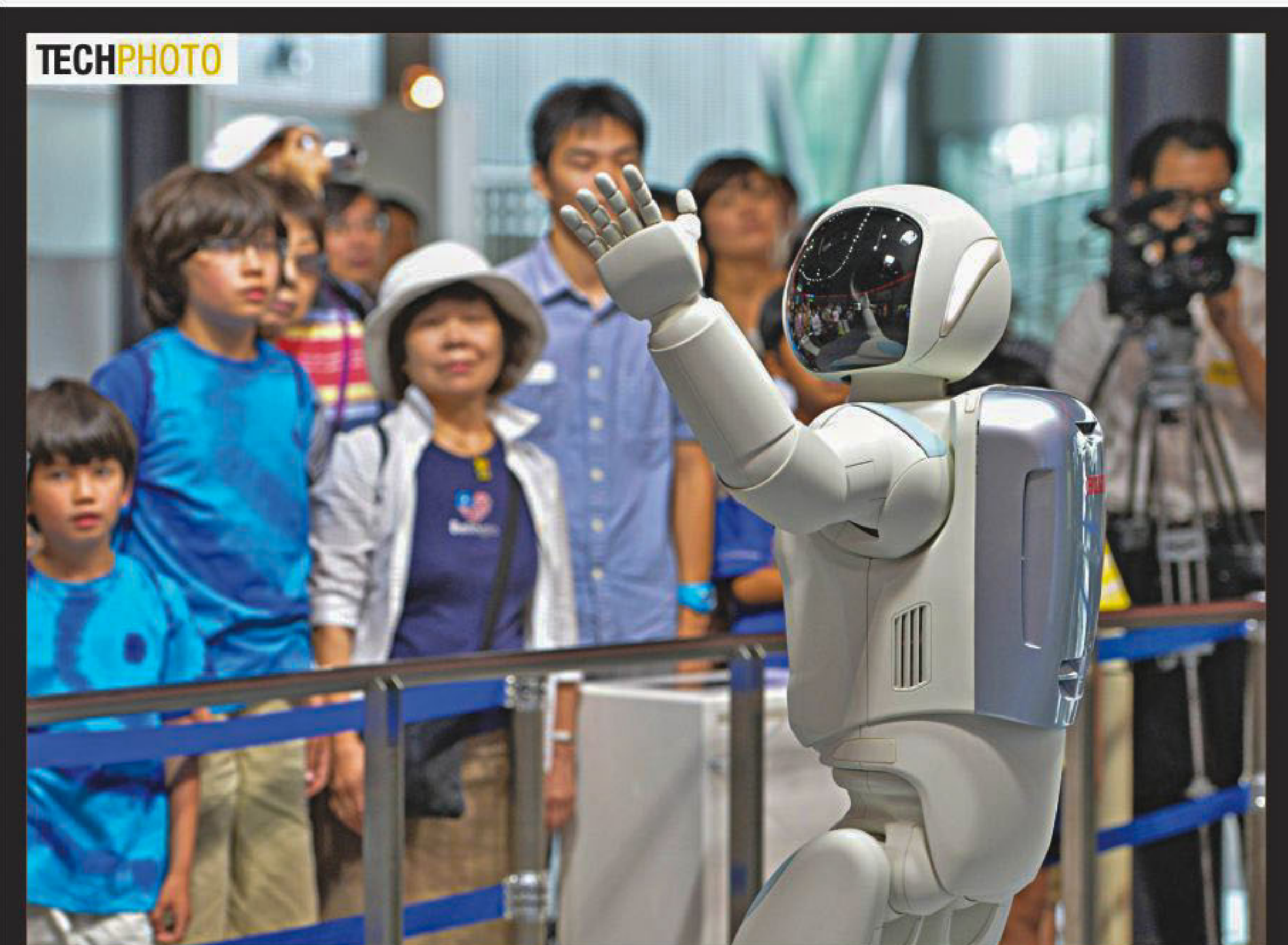
Honda Motor's humanoid robot Asimo interacts with visitors at the National Museum of Emerging Science and Innovation in Tokyo on July 3. Honda developed an autonomous behavior control technology, which enables Asimo to make decisions required to behave in concert with the movements of the surrounding people without being controlled by an operator.
