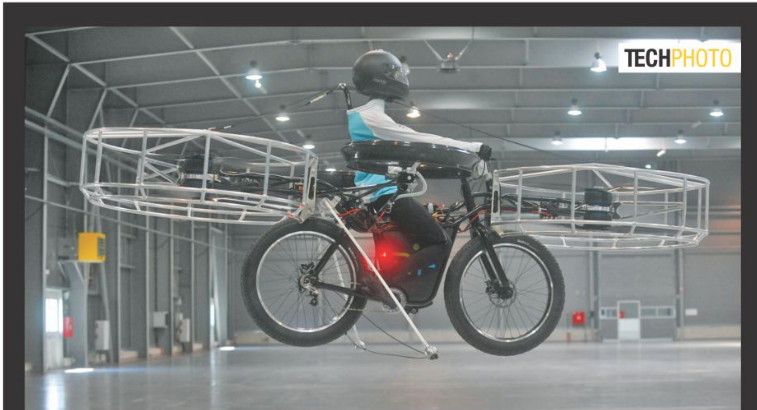
A picture taken on June 12 at the hall of Letnany fairground in Prague shows a dummy sitting on the flying bike, a unique construction of Czech designers and modern technology of French company "Dessault Systemes - 3D software tools". This bike flies thanks to six futuristic horizontal propellers and an electric motor.
