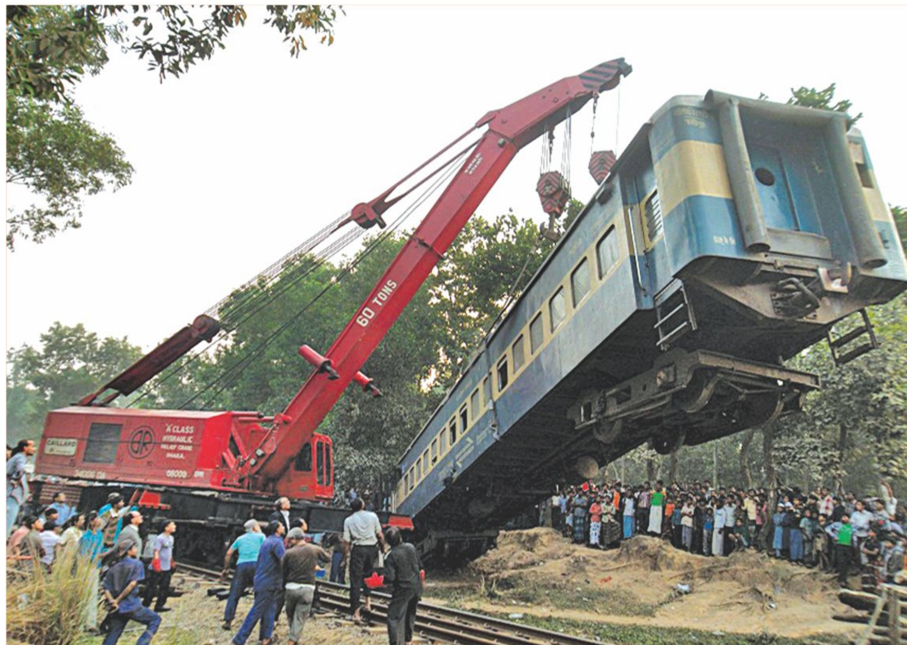
A carriage of intercity train Ekota Express being hoisted off the tracks near Matikata railway crossing in Gazipur yesterday after it lost an axle. PHOTO: STAR
