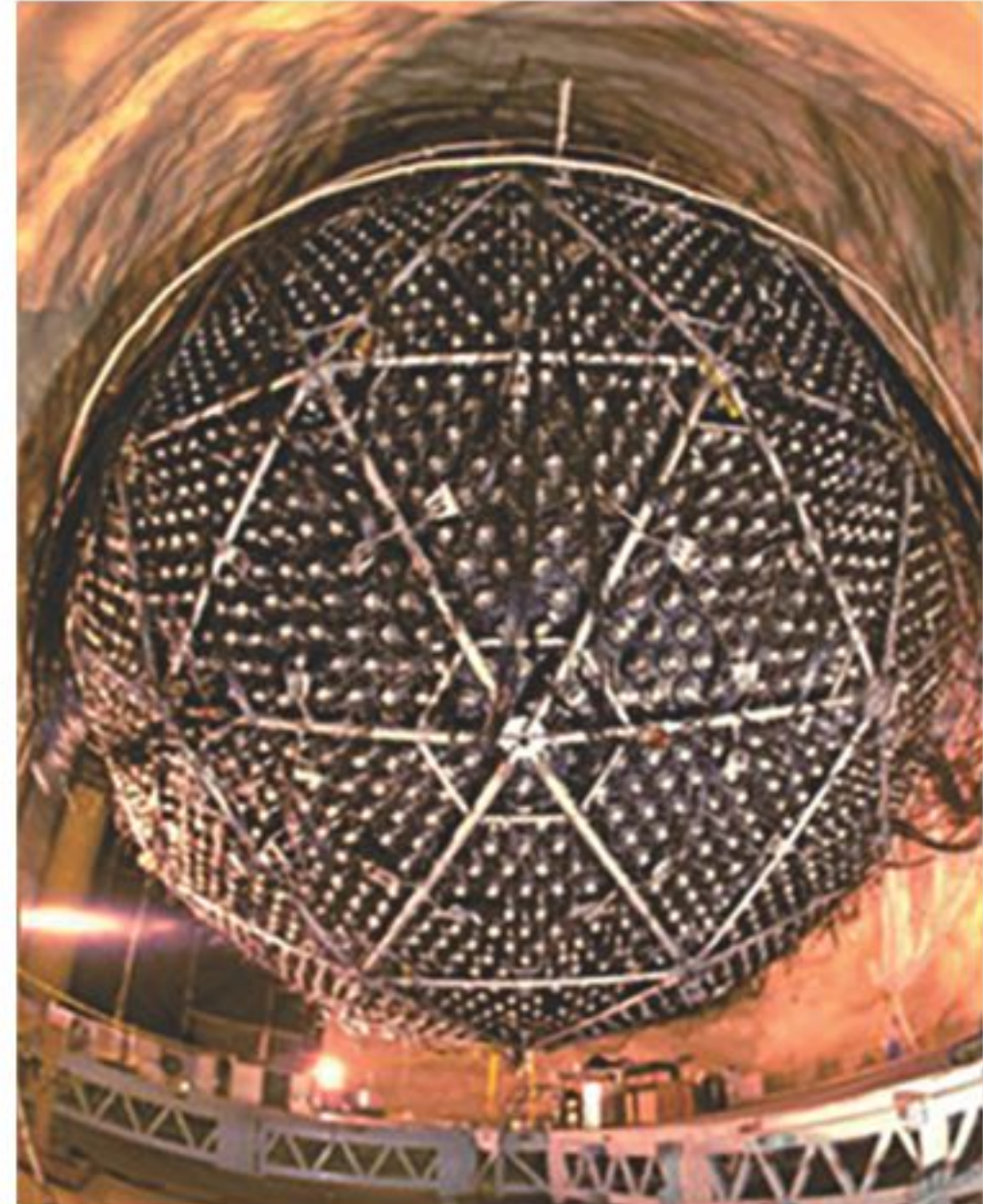
Neutrino detector buried in a nickel mine in Sudbury, Canada.
