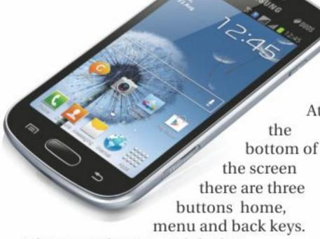
The power button and the hotswappable microSD card slot are placed at the right side while volume controller is on the left side.
