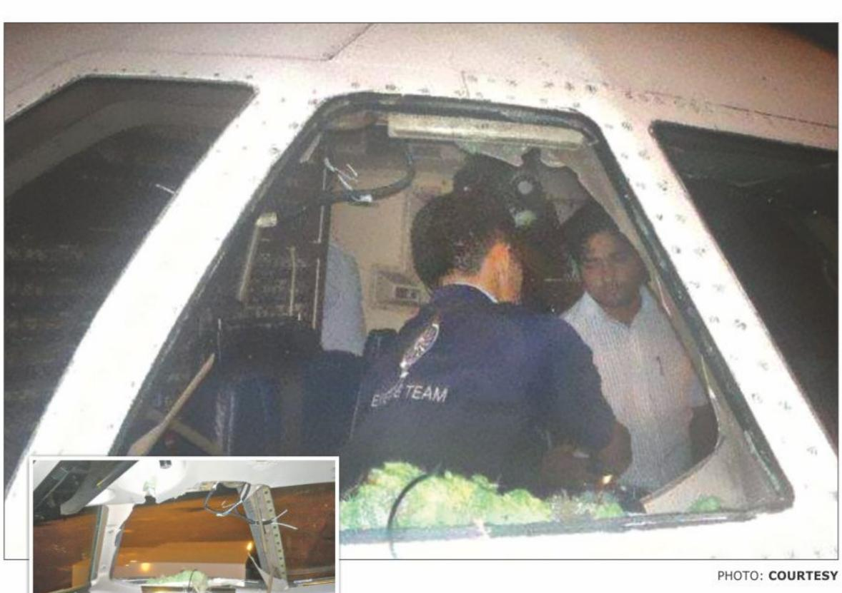
The cockpit and the frame that lost the windshield in mid-air. Luckily, the pilot managed to land the plane safely.
