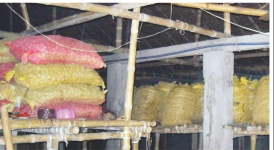
**Potatoes** stacked inside the innovative cold storage developed by **Dilip Kumar** Saha, right, the water layer under the floor that maintains moisture inside the clay-made device.
