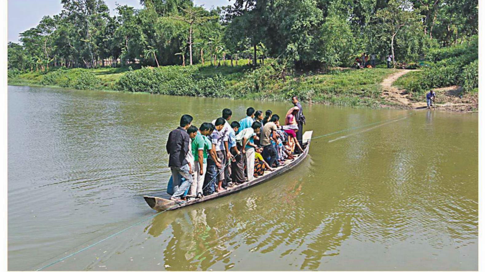
FERRY YOURSELF: The boat does not have a boatman but ferries people across the canal of Ichhamoti regularly and every passenger is charged Tk 2 for each trip. In this self-help ferry service, boat riders are required to pull on a rope fastened to either bank to propel the boat towards the other side. The photo was taken at Rangunia of Chittagong recently. PHOTO: ANURUP KANTI DAS
