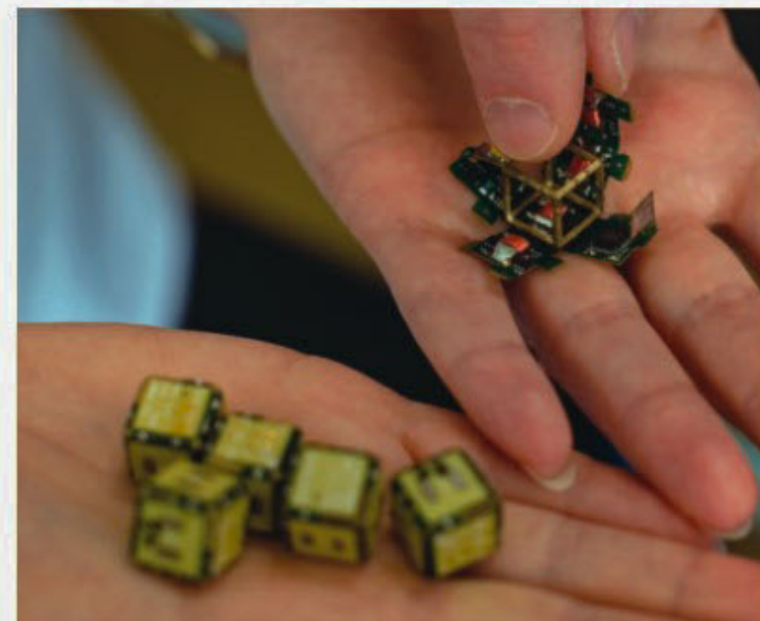
The MIT team have built test modules with microprocessors and magnets to prove their theory.
