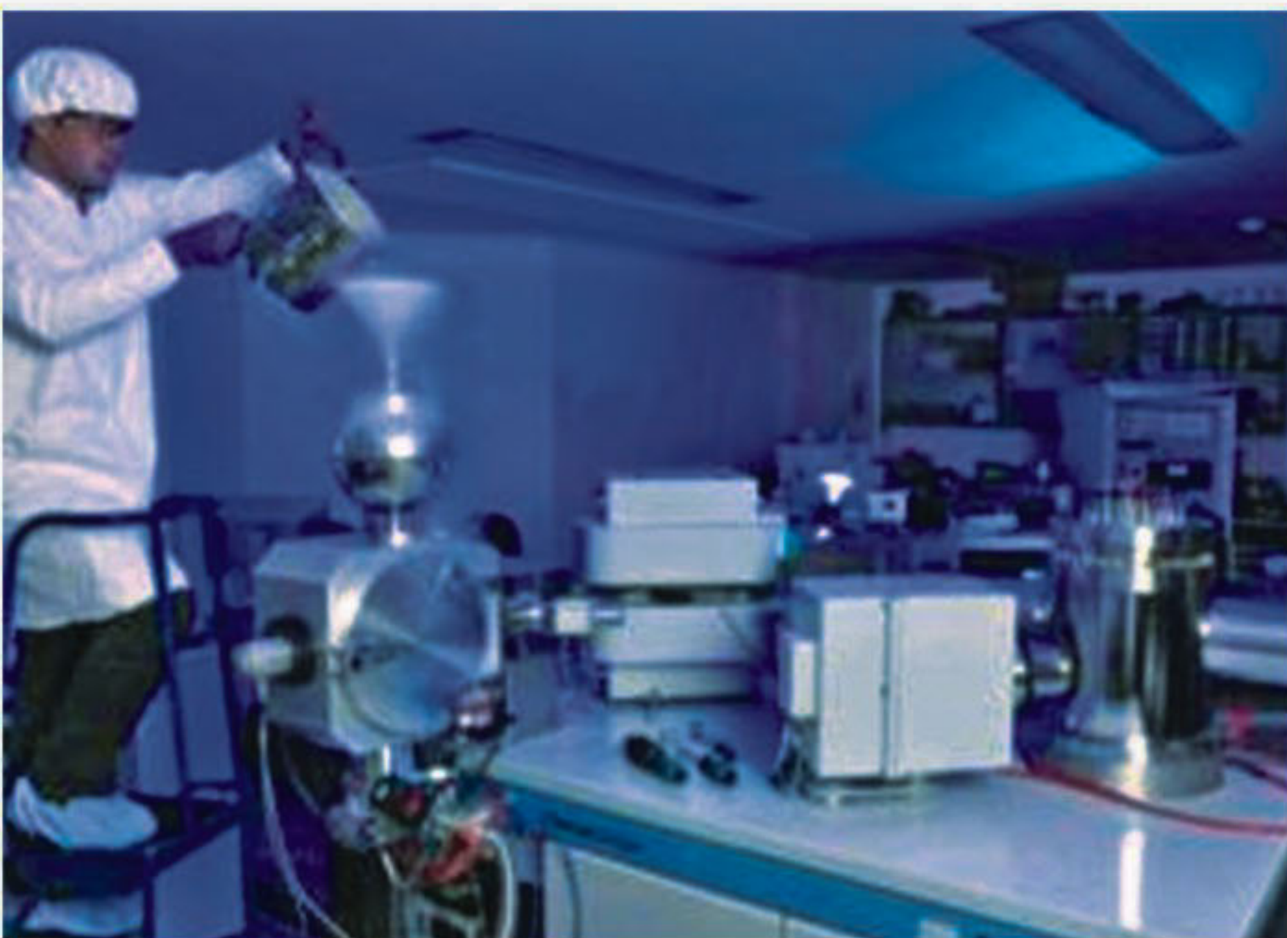
238U/235U is measured with a mass spectrometer.
