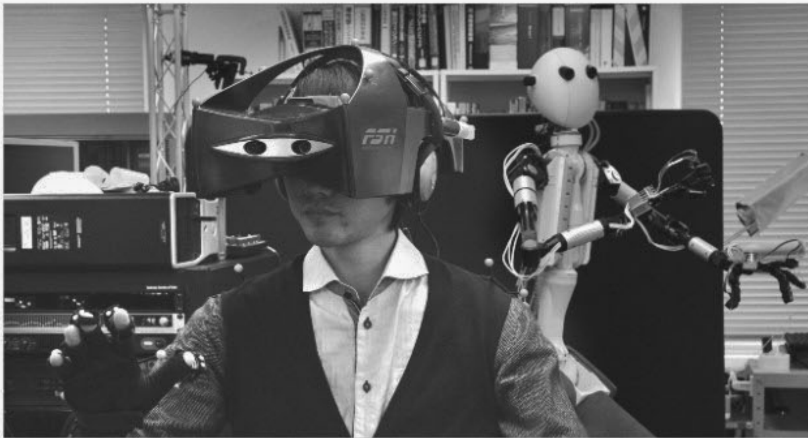
An operator, wearing a special HMD and a pair of gloves, controls a master-slave robot.
