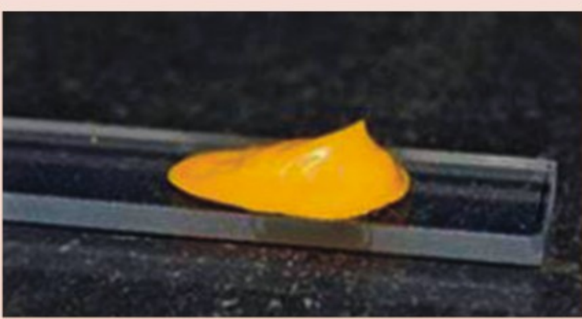
This paste of cadmium sulfide-coated titanium dioxide nanoparticles could turn large surfaces into solar cells
