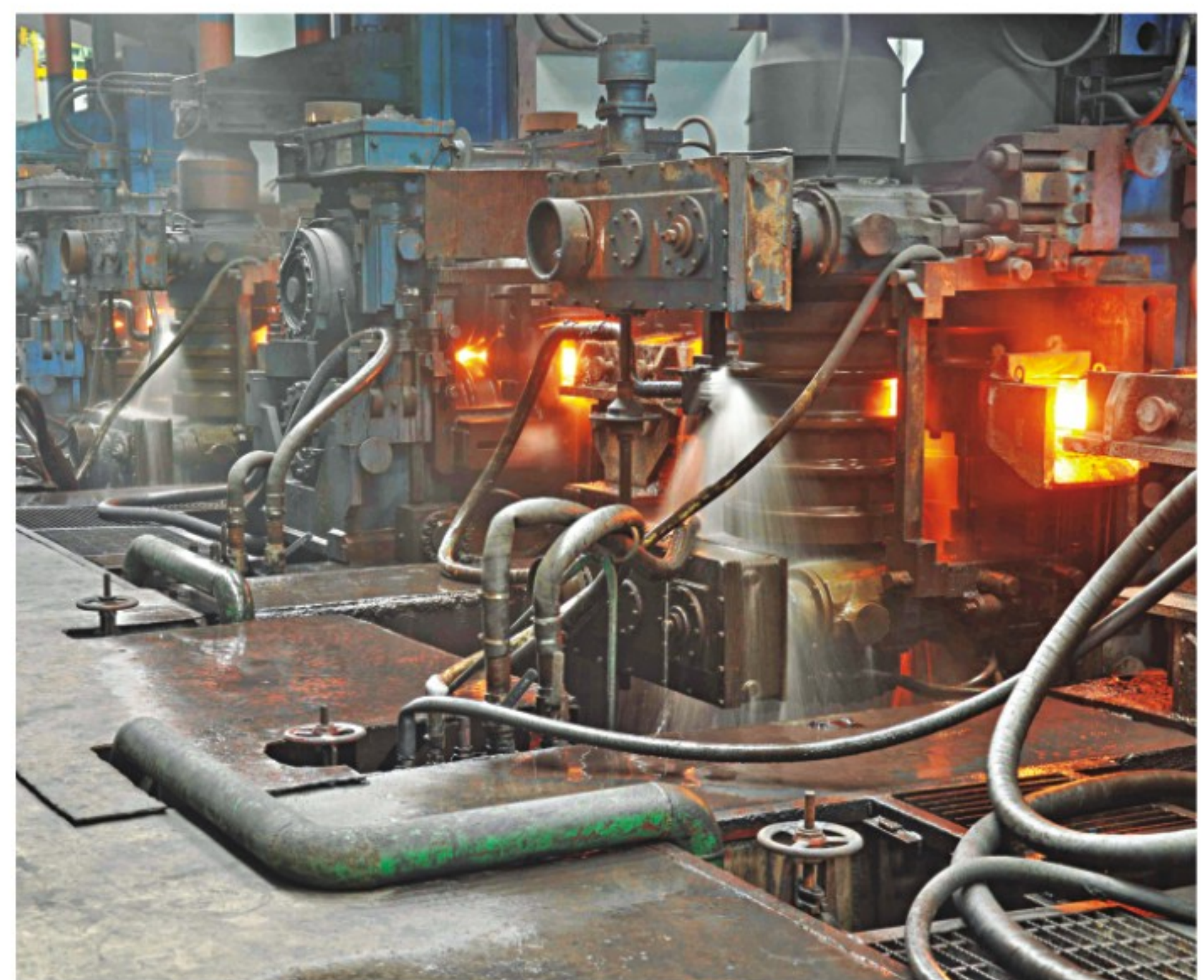
Rolling mill stand in production
