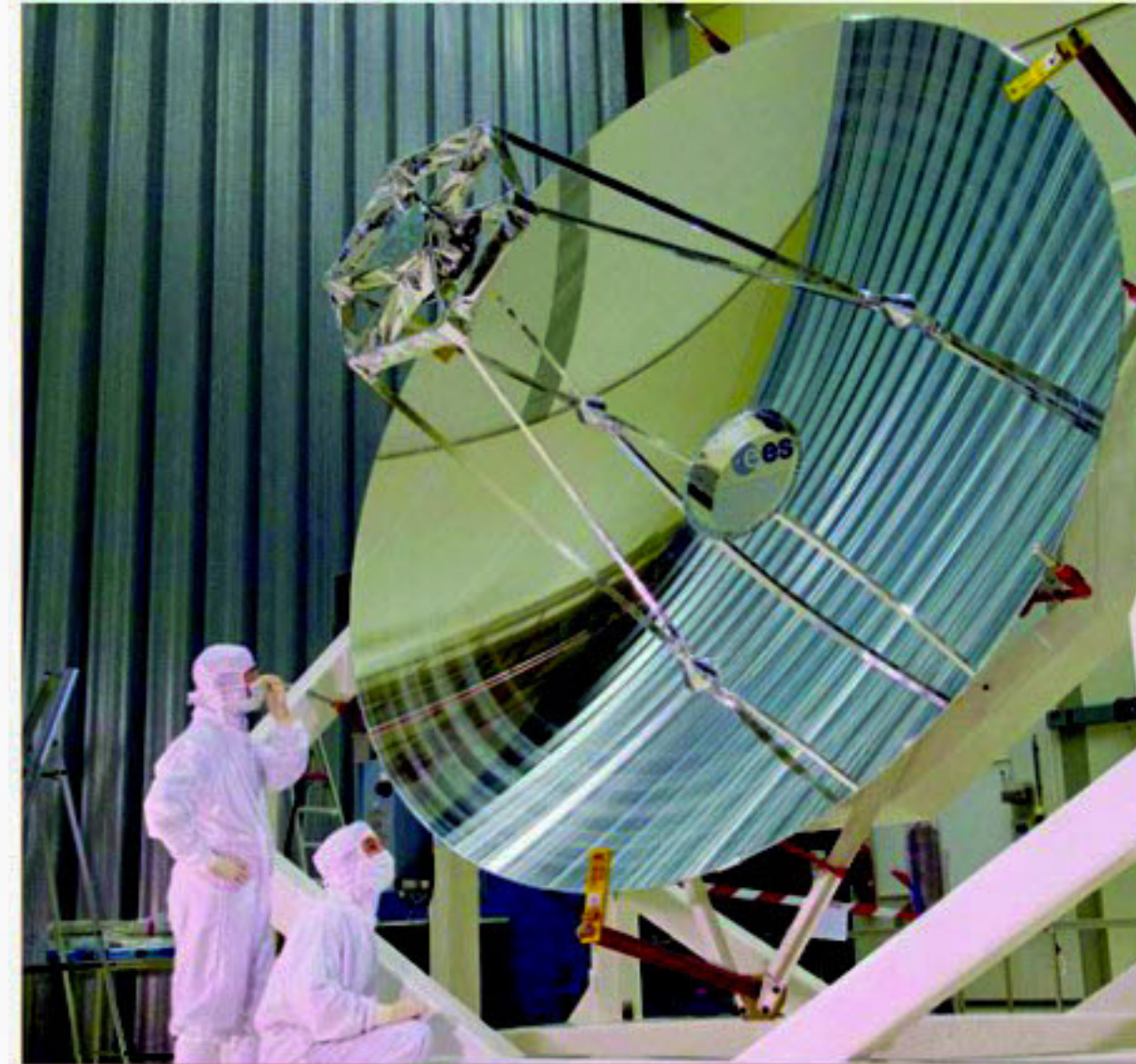
The European Space Agency's Herschel Space Observatory (formerly called Far Infrared and Submillimetre Telescope or FIRST) has the largest single mirror ever built for a space telescope.
