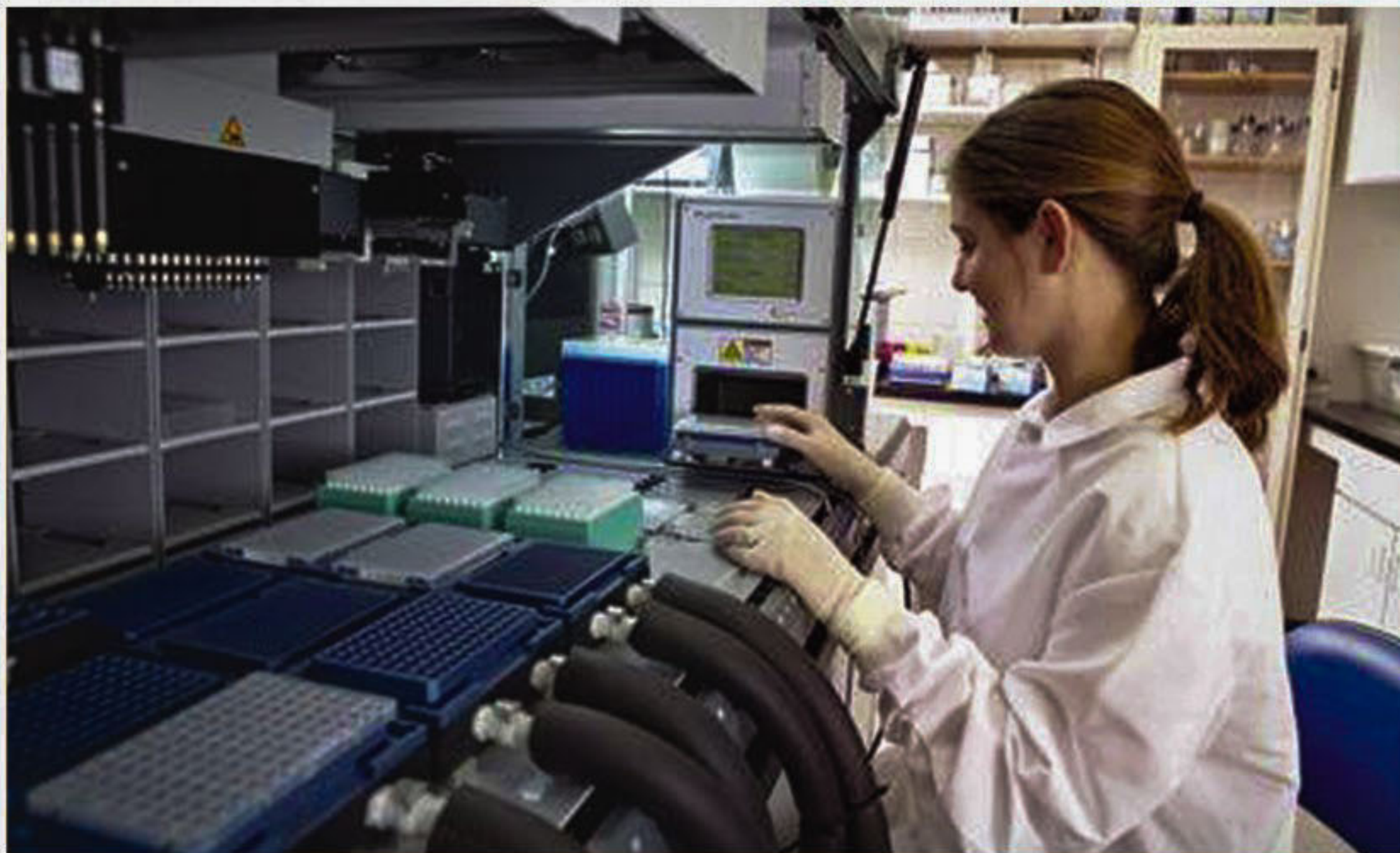
Bigelow's Dashiell Masland working with a Tecan Freedom EVO robotic liquid handler
