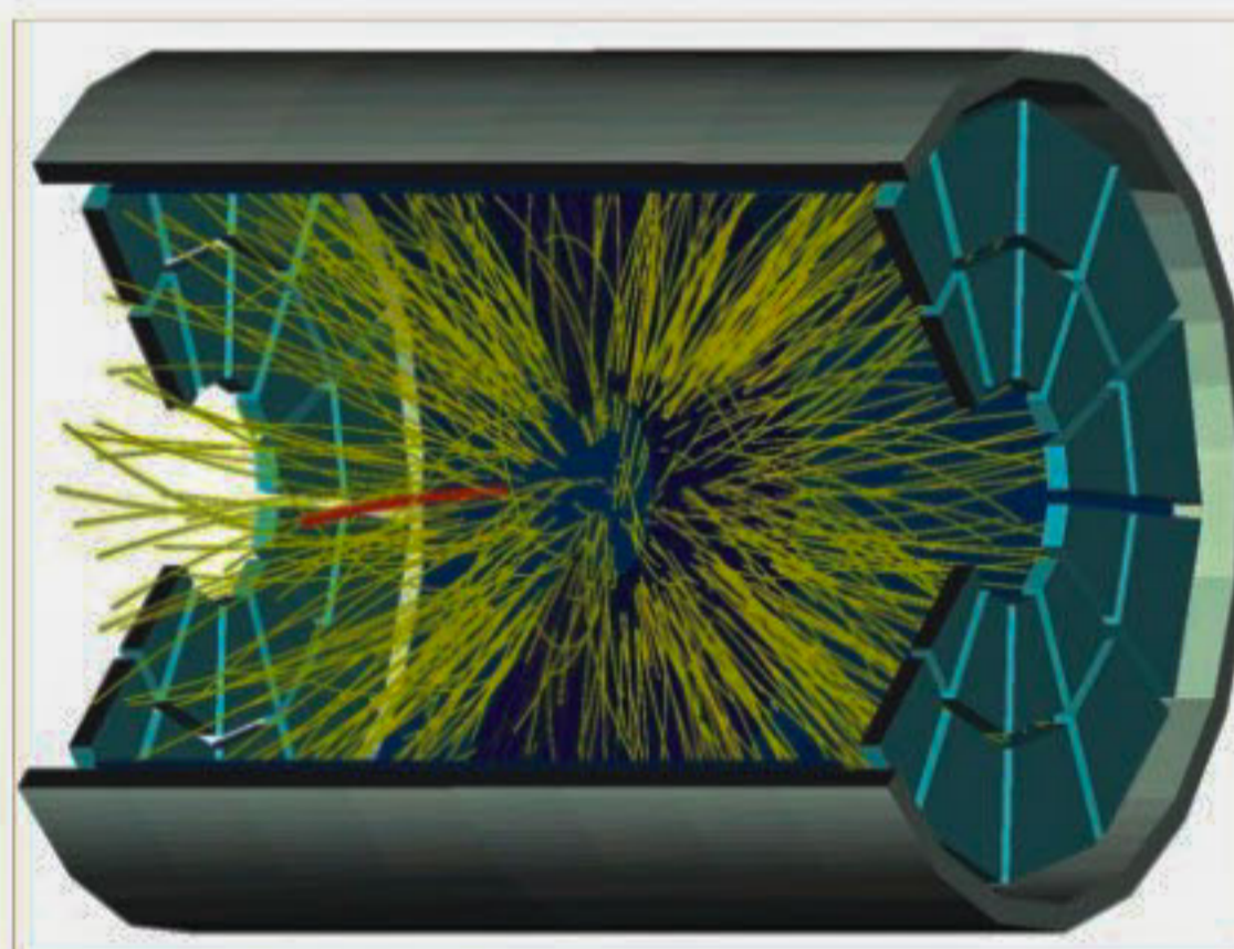
A 3D rendering of the STAR time projection chamber surrounded by the time-of-flight barrel shown as the outermost cylinder
