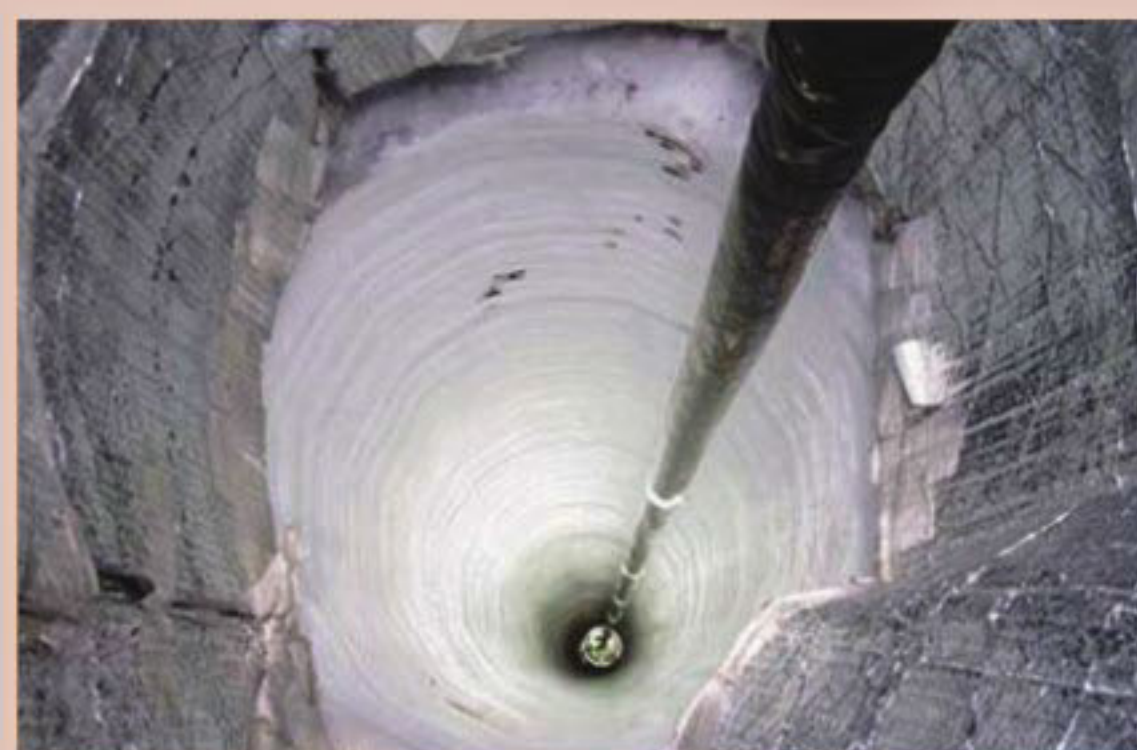
Scientists completed the largest neutrino detector with the lowering of the last of more than 5,000 neutrino sensors into holes (one shown) bored deep into the Antarctic ice sheet with hot water drills
