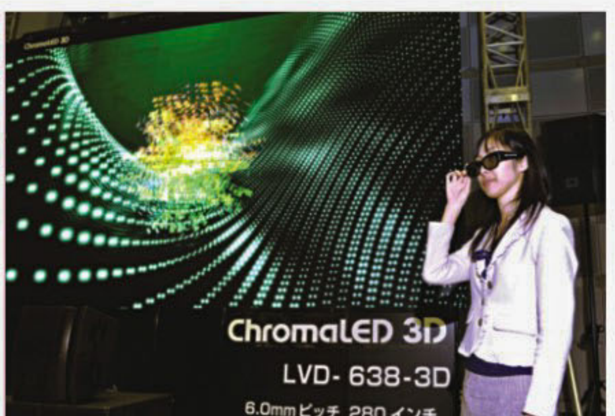
A woman puts on special glasses as Japanese electronics venture Hibino and Victor Company Japan (JVC) unveil a 280-inch sized 3D LED display, Chroma LED 3D, measuring 6.1m x 3.5m, in Tokyo yesterday. The large 3D display, using JVC technology for 2D to 3D conversion, was developed for digital signage and public viewing.
