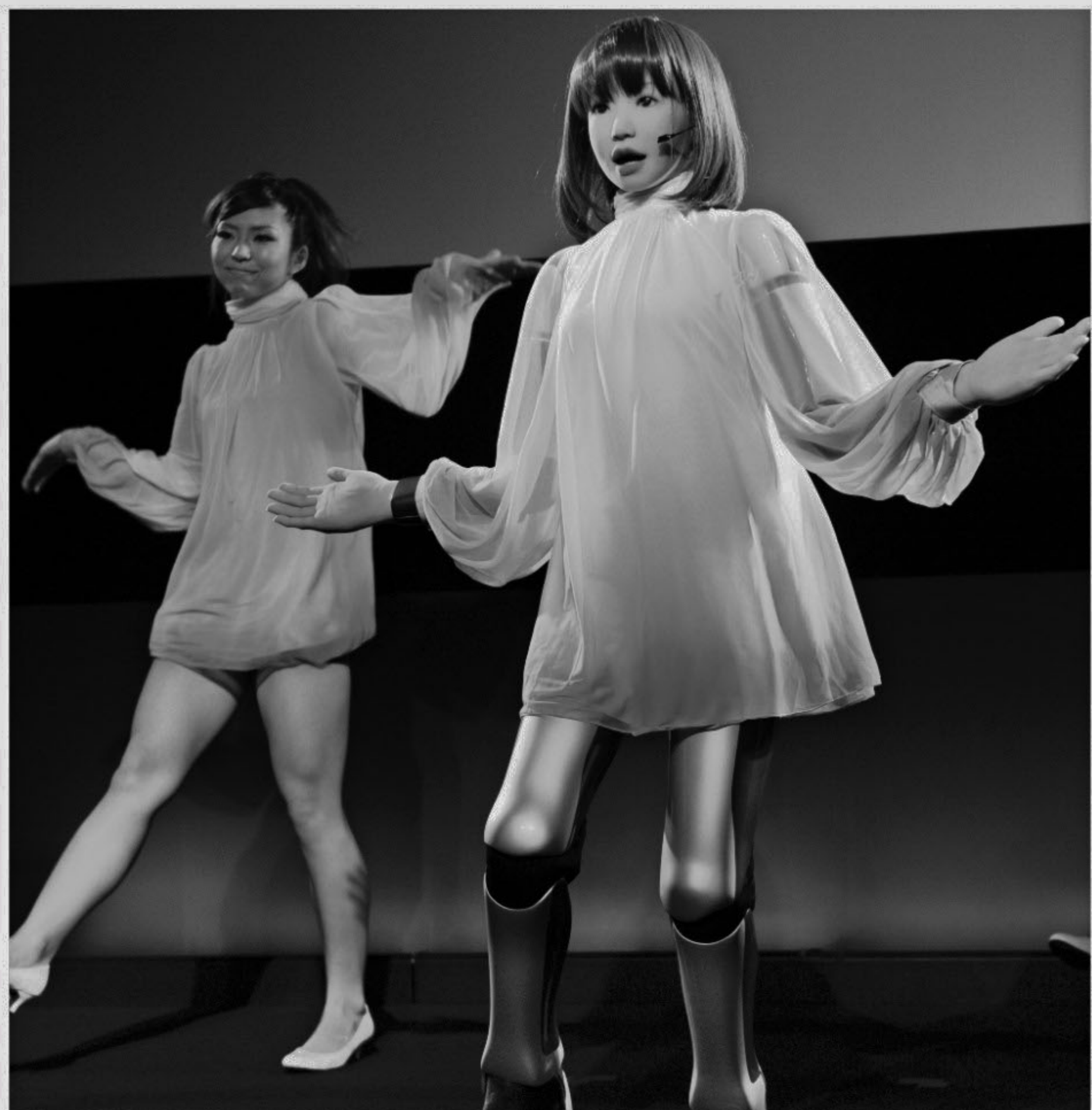
A 1.58m tall humanoid robot "HRP-4C" of Japan's Advanced Industrial Science and Technology (AIST) sings and dances with performers at the Digital Contents Expo in Tokyo yesterday. AIST developed the entertainment software called Choreonoid, formed from choreographer and humanoid.
