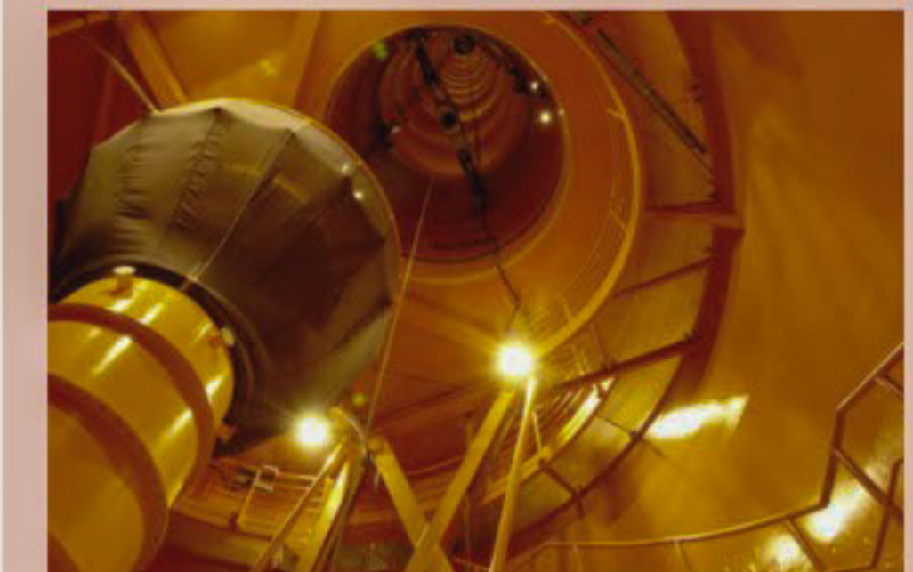
View from below, inside the 479-foot (146-meter) tall drop tower with typical experimental capsule.
