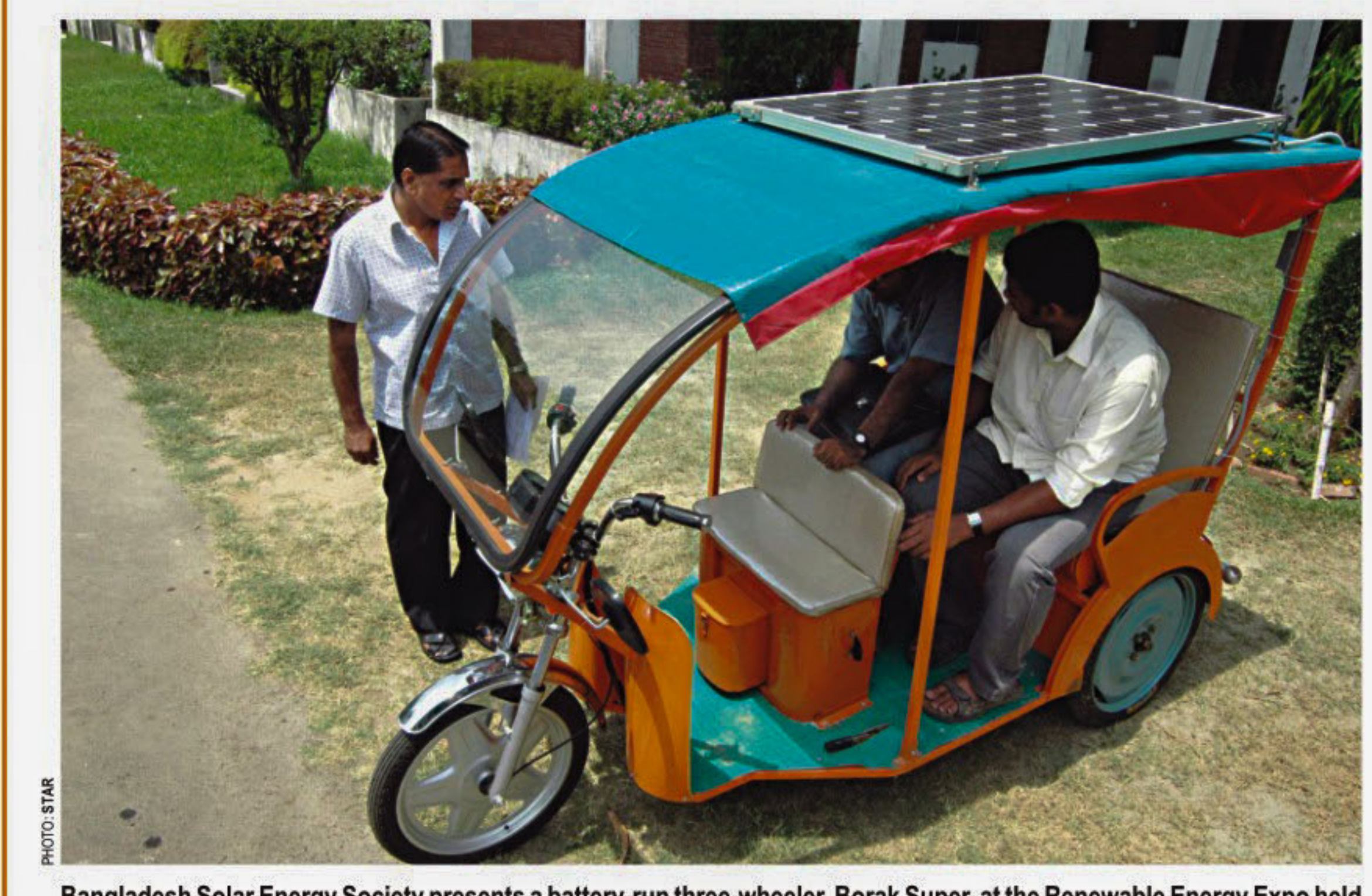
Bangladesh Solar Energy Society presents a battery-run three-wheeler, Borak Super, at the Renewable Energy Expo held in the city yesterday. A solar panel is installed on the roof of the vehicle to provide about 20 percent recharge for its batteries.
