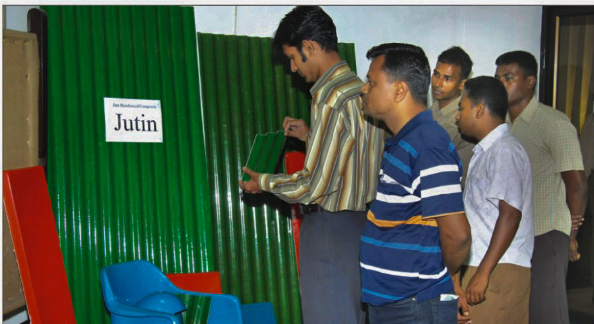
People take a look at a 'Jutin' sheet made of hessian cloth and formulated solution of polymer materials with 30-40 percent jute. Bangladesh Atomic Energy Commission unveiled the nonbiodegradable sheet in Dhaka yesterday.
