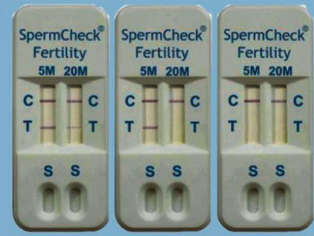
SpermCheck Fertility test devices showing expected results for normal (left), low (center) and very low (right) sperm concentrations.
