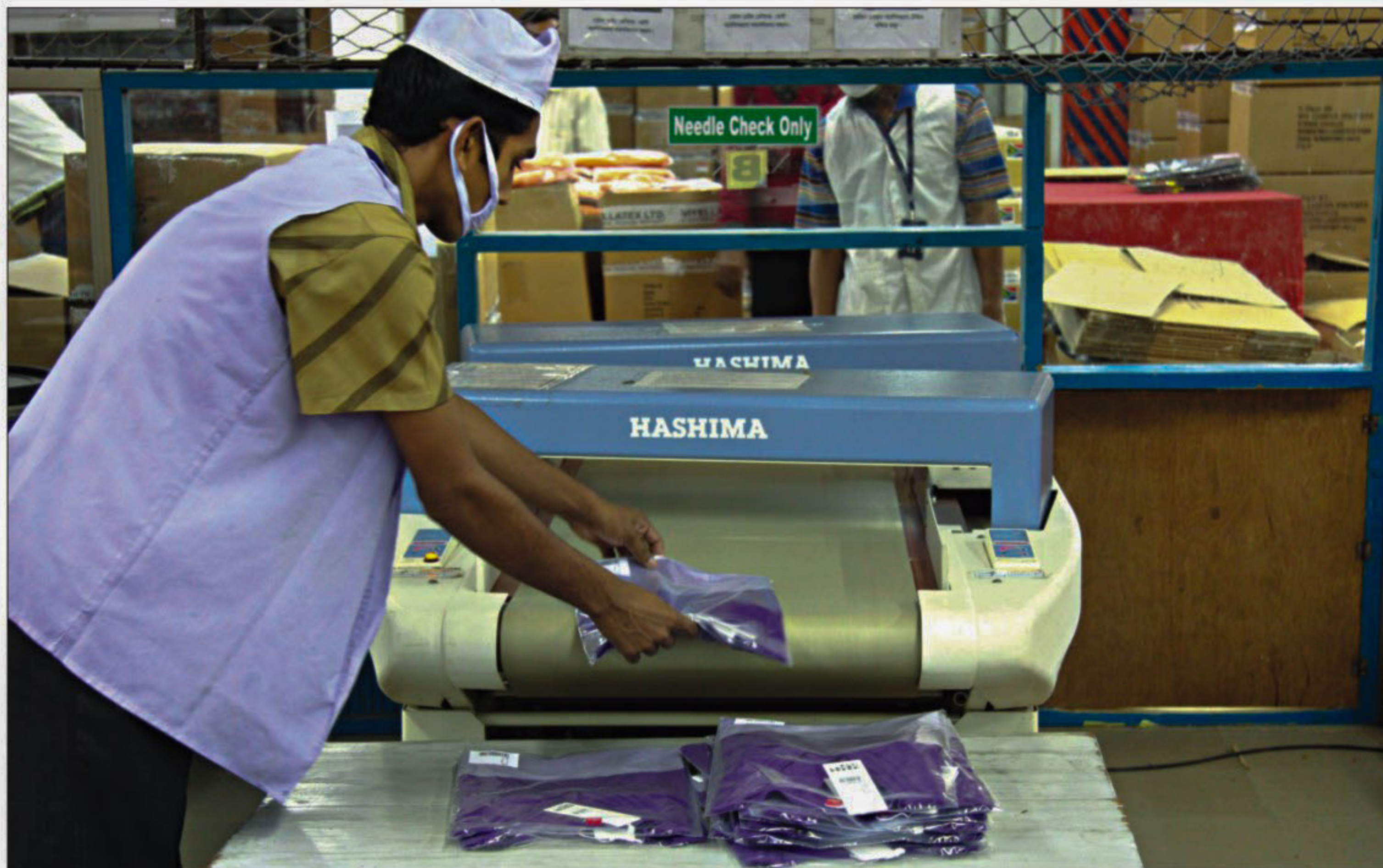
A worker runs a machine-check on garment products for needles at a factory. In the July-November period of the current fiscal year, Bangladesh exported woven garments worth $2.13 billion and knitwear items of $2.59 billion, with the share of garments in national exports increasing.
