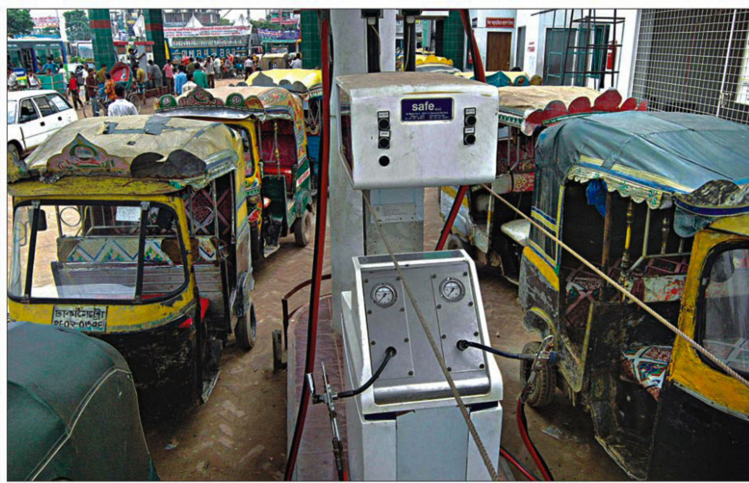
These two-stroke three wheelers were banned in the capital during the last BNP-led government's ruling, as the vehicles pollute the environment. They are now running on the city's outskirts after being converted to run on CNG. The photo was taken at Keraniganj yesterday.
