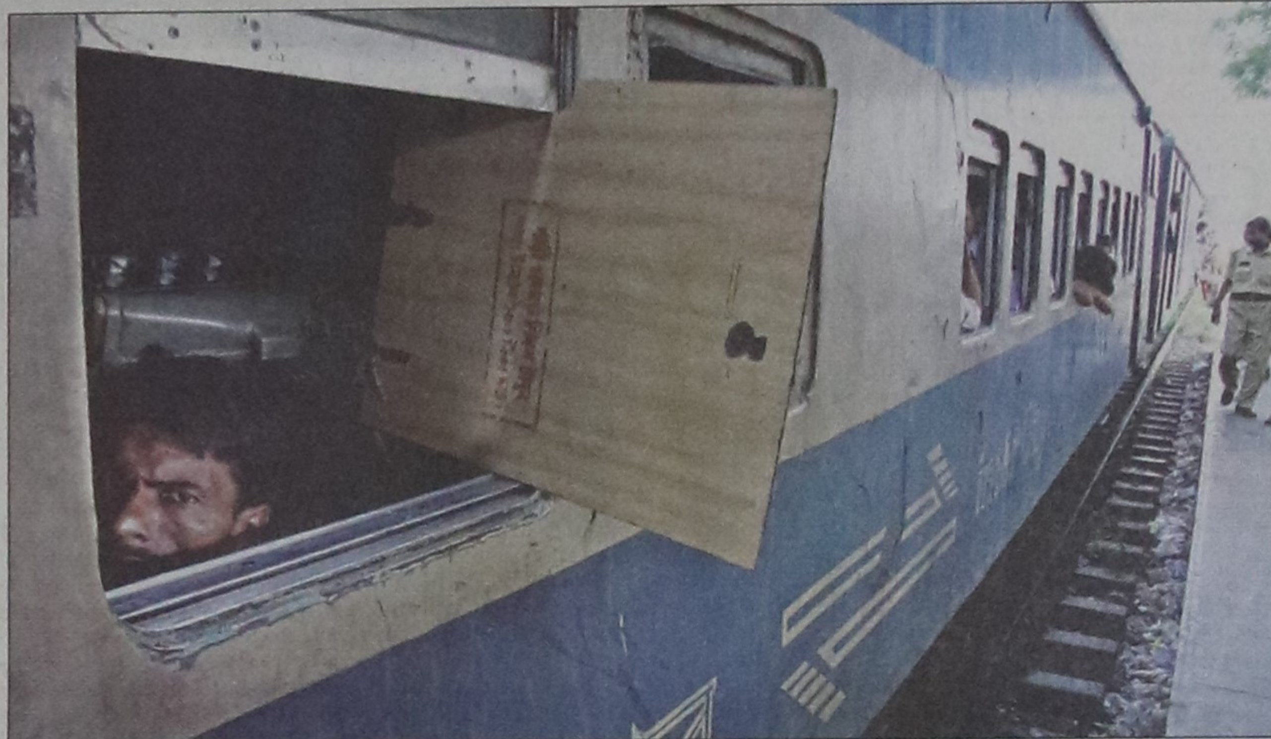
THE WIND MACHINE: As there is no cooling system inside the generator compartment of this intercity train, the engine operator set a wooden plank that flaps in the wind ensuring a flow of air into the room. The photo was taken at Tongi Railway Station yesterday.
