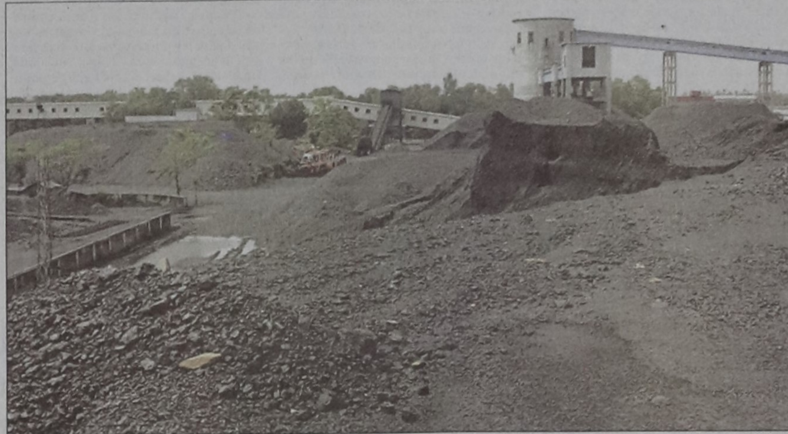
Barapukuria Coal Mine Company Limited stockpiles coal up to seven to 10 metre height at the coal yard, ignoring the international standard of piling up to three to five metres height.
