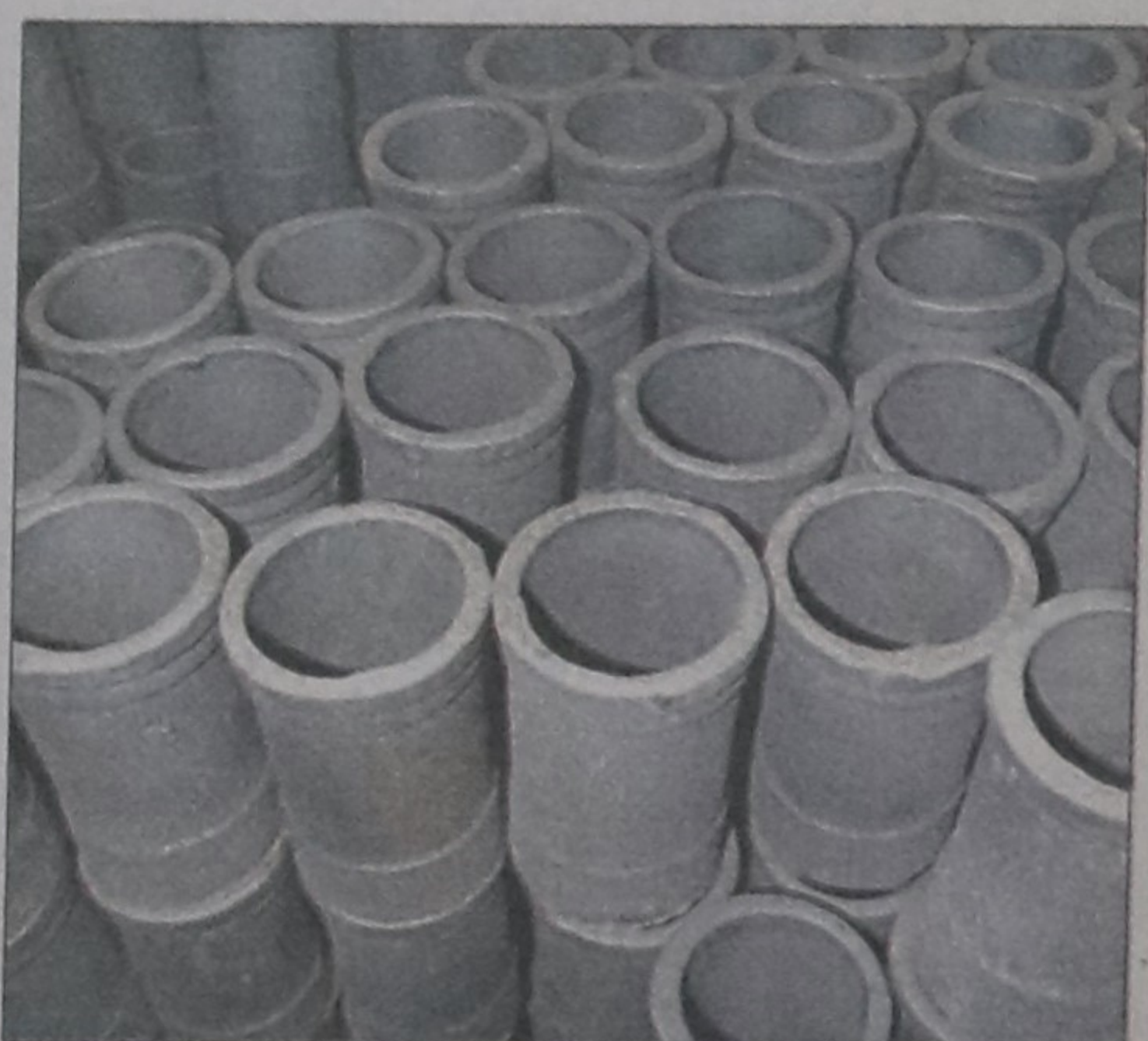
Photo shows liners made for shallow engines.
