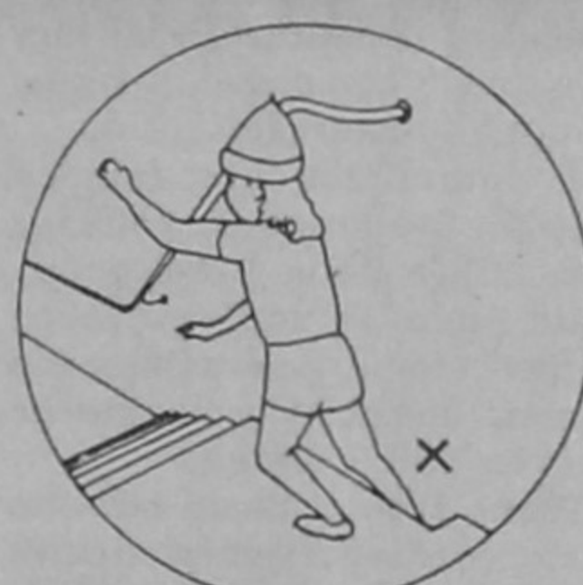
Children may fall victim to even a small gap between the flights of a stair
