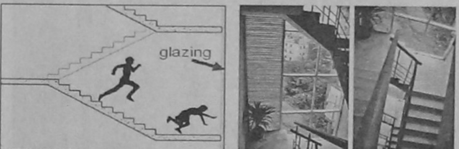
Architect's preference of style over safety: installation of fixed glazing in the danger zone.
