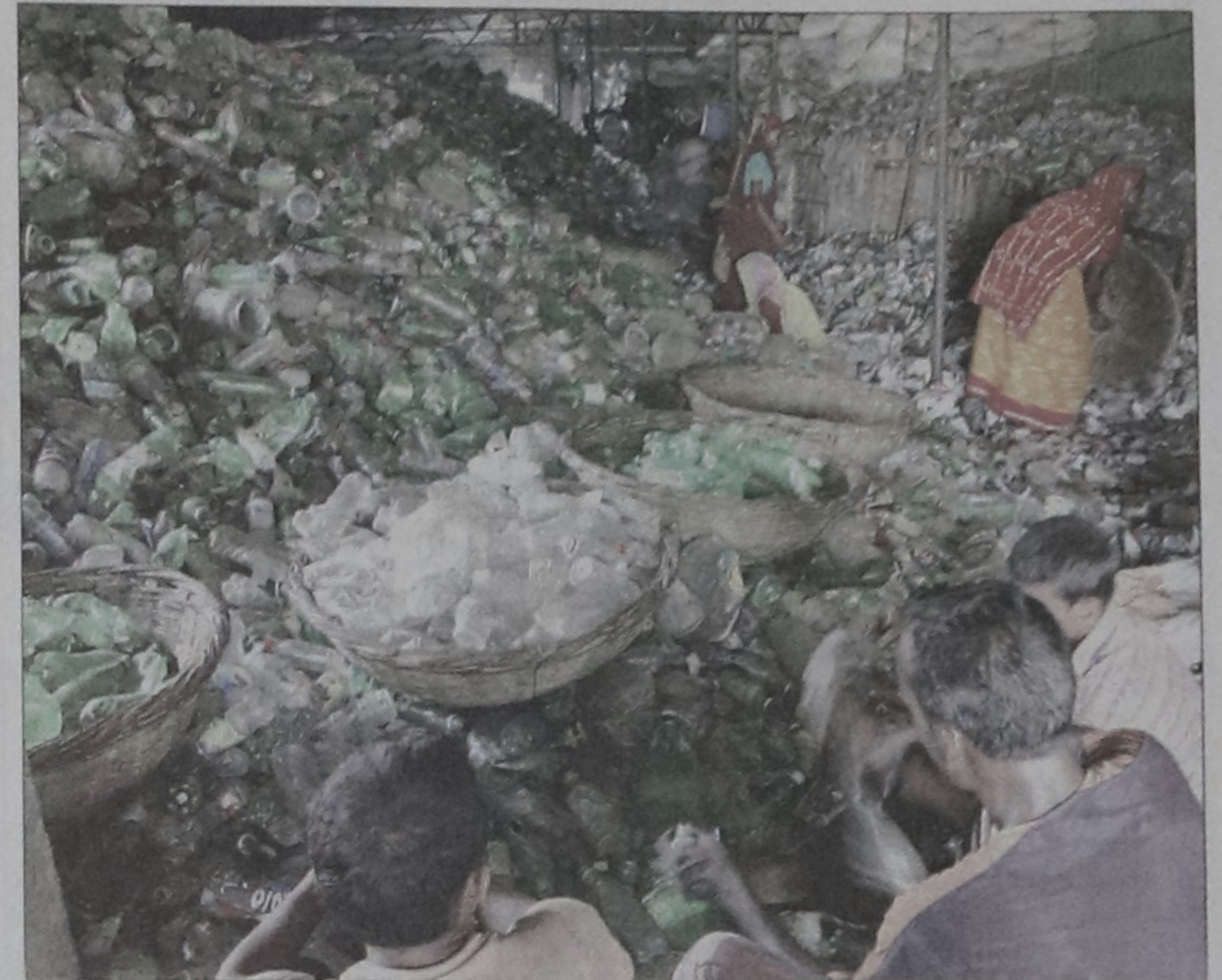
A group of workers are seen taking out the labels from the PET bottles for grinding at a factory at Savar.
