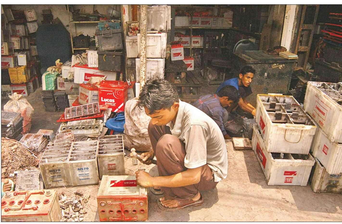
Workers are dismantling lead acid batteries in a scrap shop in Segunbagicha despite the law forbidding the activity.
