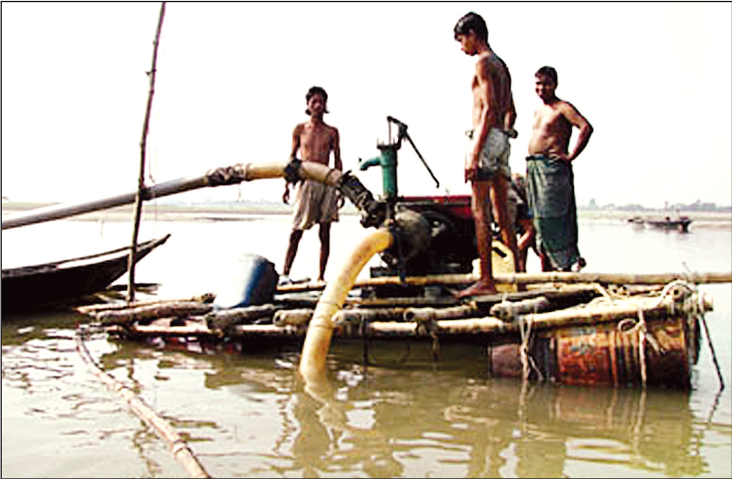
Boatmen have innovated a technique to dredge the Kalasans channel in Jamuna. They are pumping out sand by irrigation pumps mounted on makeshift raft made by joining empty drums.
