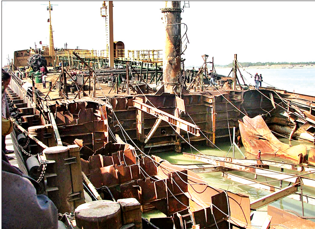
MT Banglar Shourabh, a seriously damaged oil tanker with one of its huge tank blown off, berths at Chittagong Dry Dock Limited jetty.
