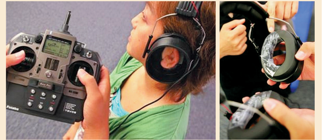
Associated Press writer Yuri Kageyama tries on a headset, left, to be remote-controlled by a technology that Nippon Telegraph and Telephone Corp., Japan's top phone company, is developing during a demonstration at an NTT research in Atsugi, near Tokyo. An earphone headset, right, is shown that sends an electric current from the back of the ears through the head.
