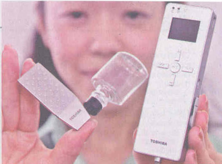
Japanese electronics giant Toshiba employee Hiroko Mochida displays a prototype model of the IC audio player, powered by direct methanol fuel cell (DMFC) battery unit (L) which enables to play 35 hours with a single 3.5ml charge of methanol at the company's headquarters in Tokyo. Toshiba developed two prototype fuel cell units that would realise extended playing time for mobile music players and will be commercialised in 2007.
