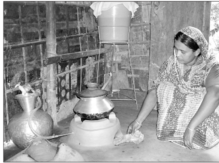
Household installation of Chulli water purifier
