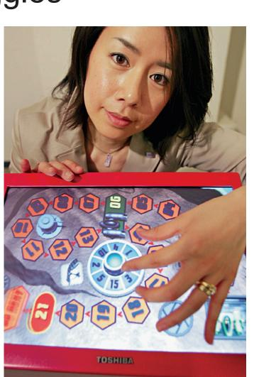
Japan's electronics giant Toshiba researcher Rieko Fukushima displays a prototype model of the new flatbed type three-dimensional (3D) LCD display without special glasses, which enables to show 16 different angles 3D images with a technology of integral imaging system employing semicylindrical micro-lenses on its surface at the company's headquarters in Tokyo on April 15. Toshiba is expected to put it on the market at the end of
