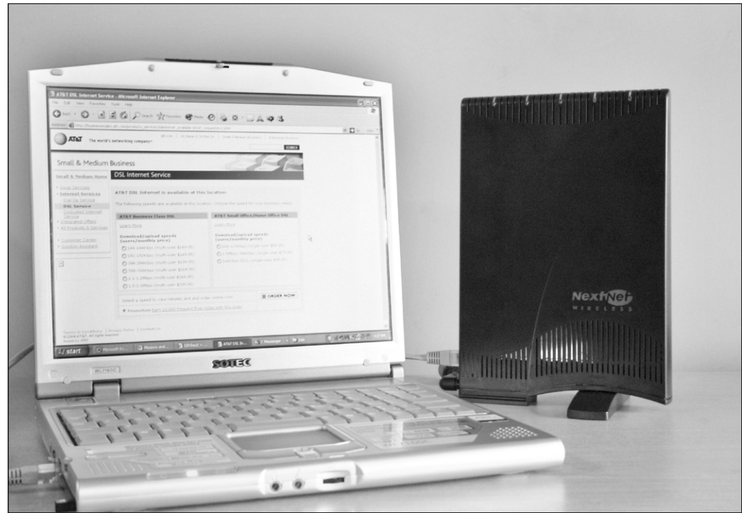
The NextNet Wireless modem used for XSTREAM NLOS
