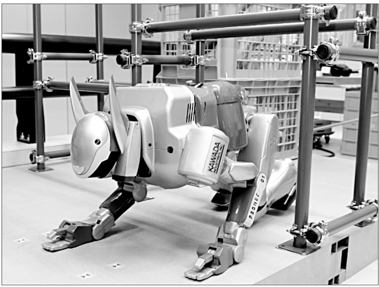
Humanoid robot "HRP-2" developed by the National Institute of Advanced Industrial Science and Technology (AIST), is prepared for a demonstration in Tsukuba on September 21. Researcher Dr. Kensuke Harada along with six colleagues at the AIST succeeded in enhancing the walk and work capabilities of the working humanoid robot standing 154cm tall and weighing 58kg.
