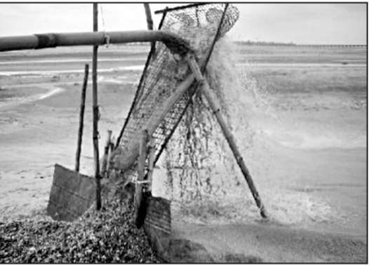
Workers engaged in collecting rock (left), a boring machine mounted on a raft made with drums extracting rocks from the river bed (middle) and rocks funneled through pipe from the river being separated from sand and water (right). The photos were taken from Chhai Anir Char on Sunday .
