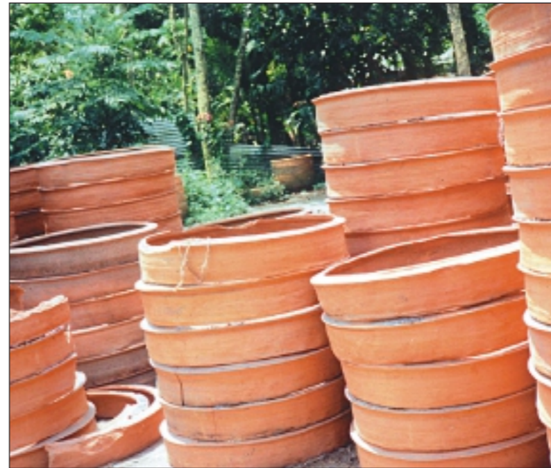
Indranath Pal, a middle-aged potter, and his wife, right, in Bamunkushia village in Tangail have stepped beyond grinding poverty by producing ring slabs of clay, left, a cheap alternative to cement slabs used for sanitary latrines.
