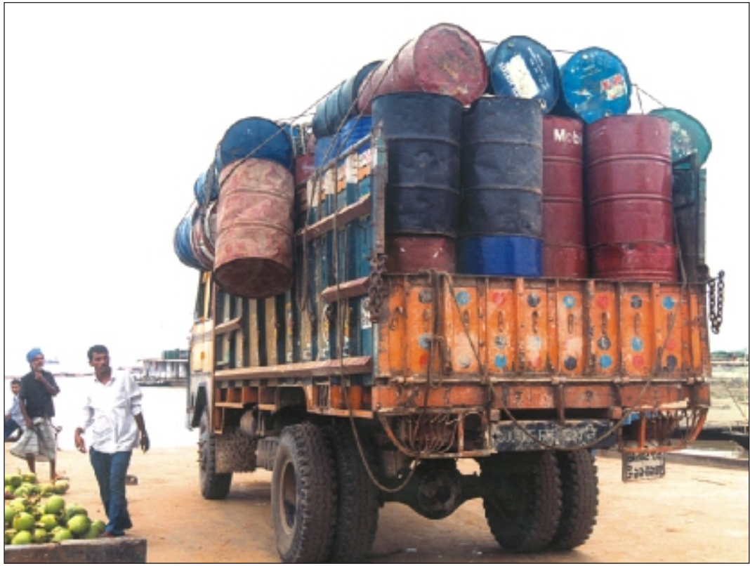
An overloaded truck bound for Paturia in Manikganj waits to cross the Padma river by ferry. Trucks packed beyond capacity are a menace to traffic on the highways and ferries. The excess weight also wears down roads fast.
