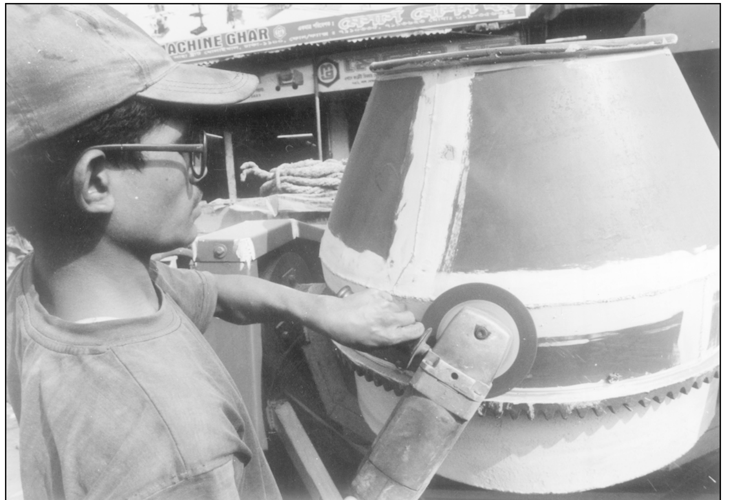
A worker gives finishing touches to a mixer machine used for making mortar for building construction at Dholakhal in Dhaka. The price of a locally made mixer machine is half of a foreign one.
