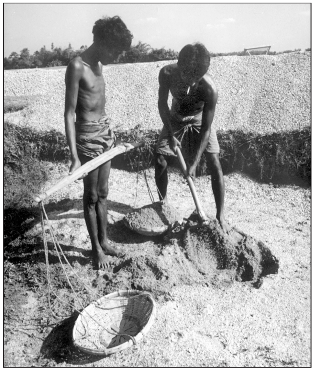
Two labourers dig ground to extract stones at Panchagarh. Stones are found abundantly in this northern district from where those are sent to other parts of the country for construction purpose.
