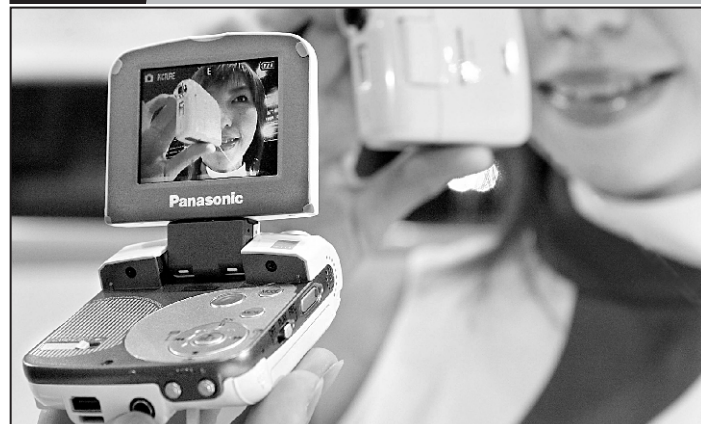
Japan's electronics giant Matsushita employee Aki Goto displays the new tiny digital camera "D-snap SV-AV30" weighing 95g and equipped with a 350,000-pixel CCD on its image sensor at Asia's largest PC trade show WPC Expo 2002 in Tokyo 16 October 2002.
