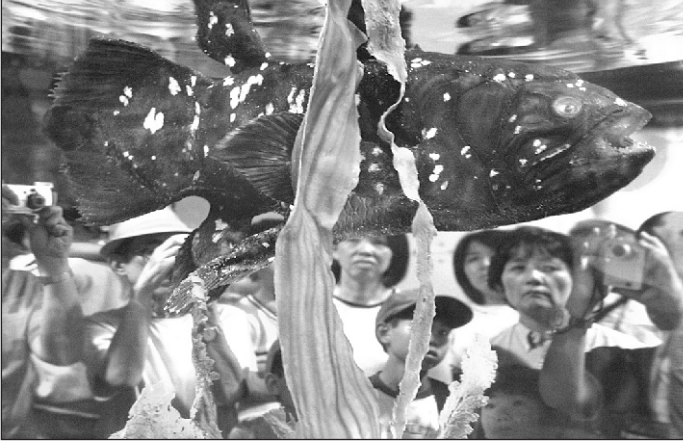
People look at a robot fish modeled after a coelacanth as it swims in a glass tank at the Japan's Mitsubishi Minatomiri Industrial Museum in Yokohama, 06 August 2002. The 80-centimeter-long robot incorporates propulsion technology Mitsubishi Heavy Industries developed for use in submarines and ships. The robot can float and use its five elastic fins to swim like a real fish.
