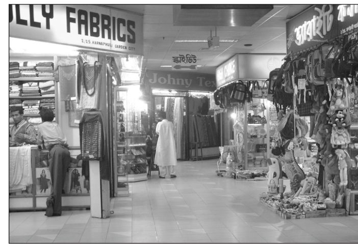
Haphazardly stored material narrows the effective width of the corridor.
