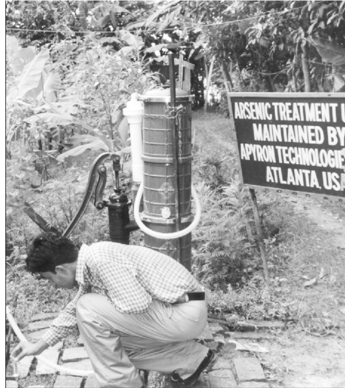
Aprylon system serves Adahata and Maricha villagers in 24-Parganas with safe arsenic-free water.
